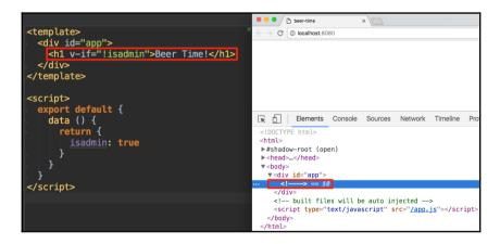
Conditional rendering using the v-if directive. Condition is not met.
