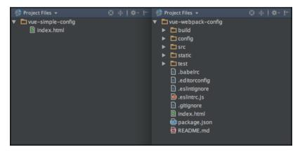
The difference in structure in application scaffolded with vue init simple and vue init webpack
