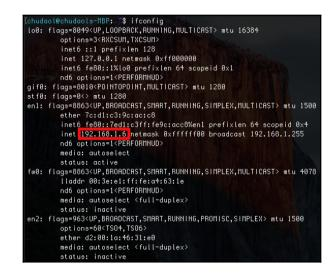
Checking the IP address with the if config command
